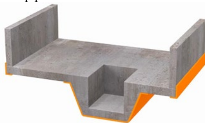
Pic. 1. The side of a foundation slab and an elevator shaft pit waterproofed with Hydrostop-Penetrating Mat.
