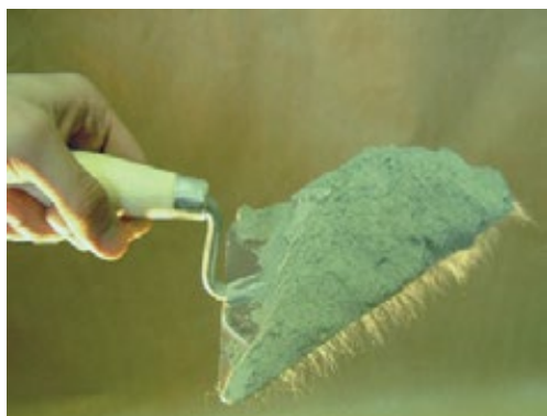
Fot. 1. The appearance of dry Hydrostop-Repair with visible polypropylene fiber.
